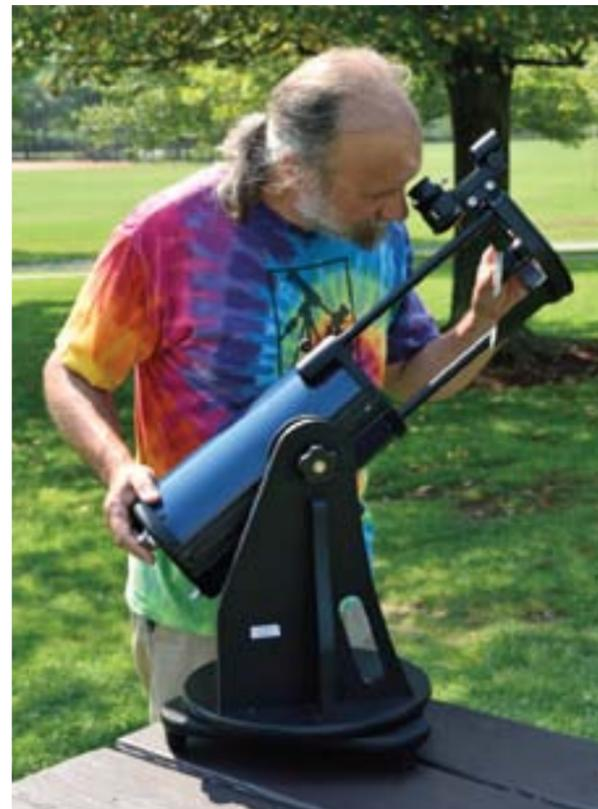
The OneSky works best on a standard-height table or similar support. The telescope focuser's fixed position forces users to stand behind the instrument when viewing near the zenith.
