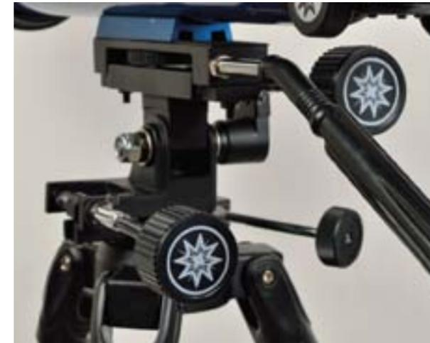
**Roughly aiming the Meade Infinity 90 refractor is aided by using the long handle at the back of the tripod. Targets can then be centered with the slow-motion controls.**
