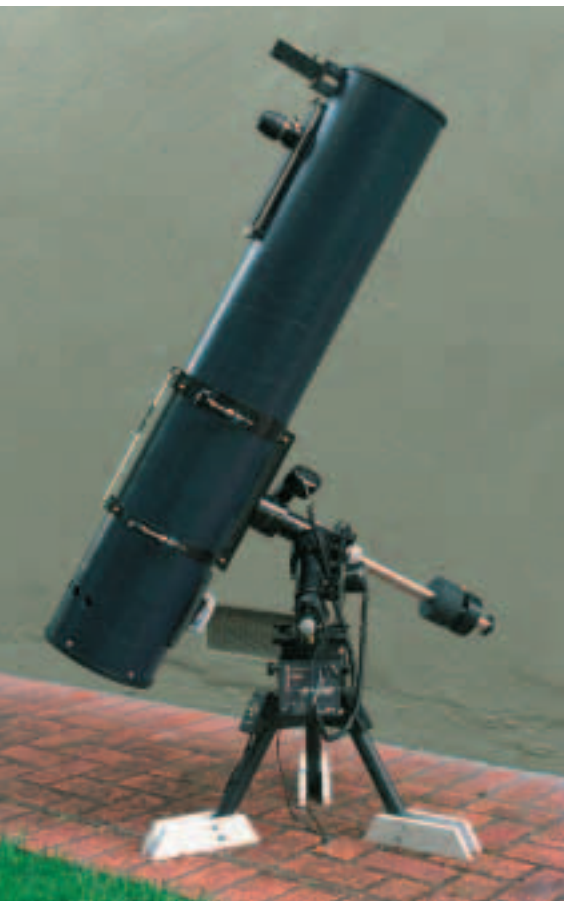
An overview of Adler's high-performance 8-inch f /6 Newtonian, which features a spherical primary mirror flexed into a superb paraboloid. Except where noted, all illustrations are courtesy the author.
