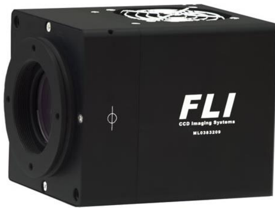
Figure 4. The Finger Lakes Instrumentation Microline ML8051 camera uses 12MHz digitizing speed for a fast frame rate with low readout noise. The interline CCD sensor does not require a mechanical shutter, so vibrations and delays are minimized.
