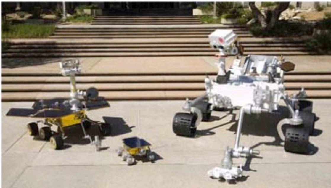
Weighing about a ton, the rover Curiosity (right)) is far larger than its predecessors Spirit and Opportunity (left)), which reached Mars in 2004; and tiny Sojourner (center)), which landed in 1997. NASA / JPL
