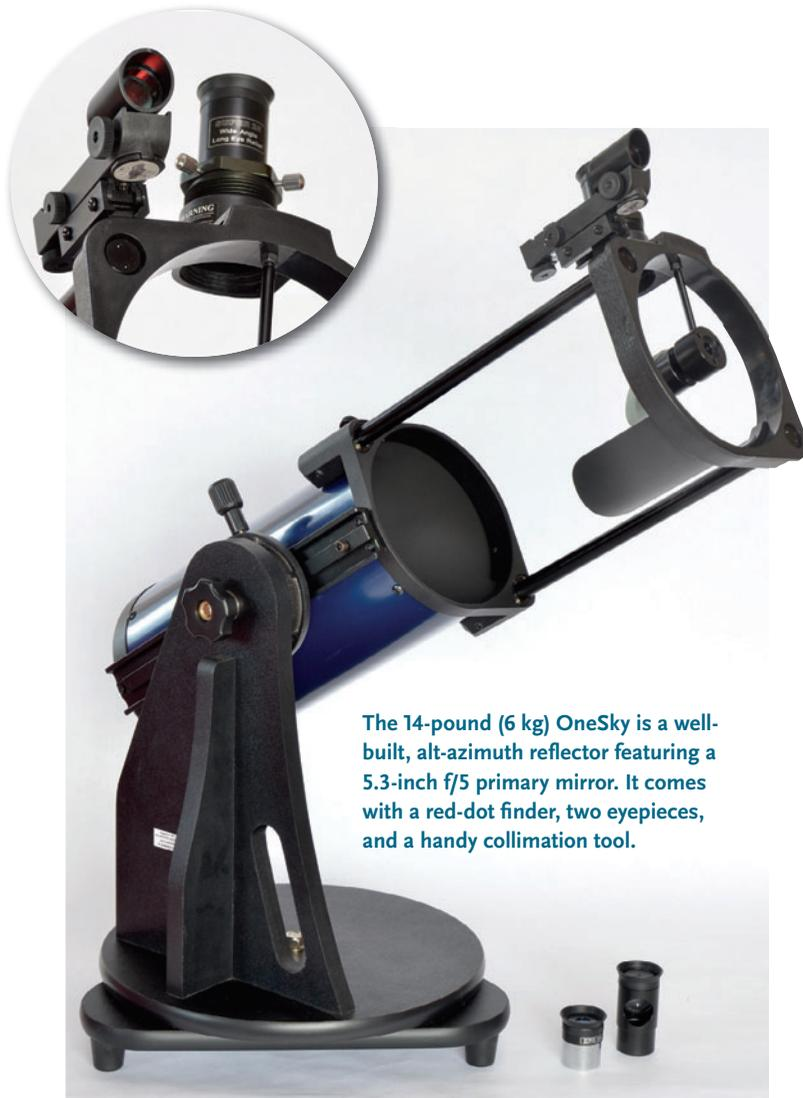
The 14-pound (6 kg) OneSky is a well-built, alt-azimuth reflector featuring a 5.3-inch f/5 primary mirror. It comes with a red-dot finder, two eyepieces, and a handy collimation tool.
