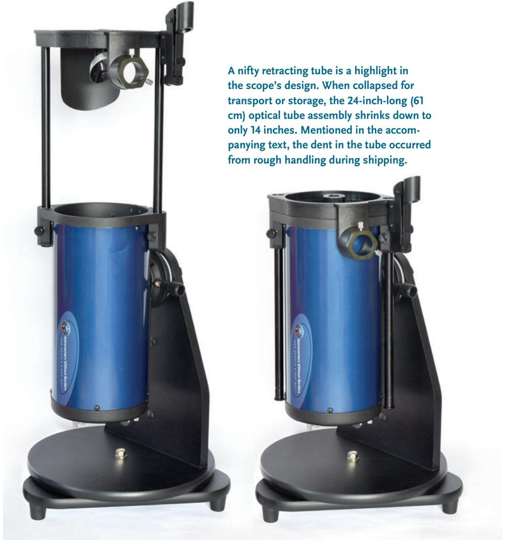
A nifty retracting tube is a highlight in the scope's design. When collapsed for transport or storage, the 24-inch-long (61 cm) optical tube assembly shrinks down to only 14 inches. Mentioned in the accompanying text, the dent in the tube occurred from rough handling during shipping.
