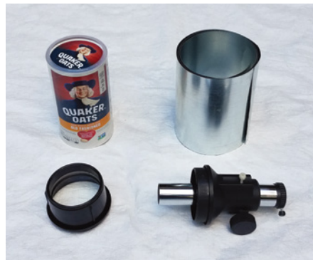
▲ Making your own refractor requires the lens, the focuser, a tube to hold them the right distance apart, and a dew shield.
