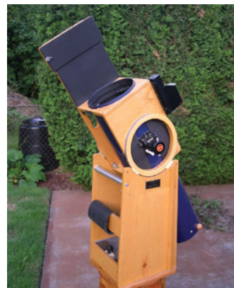
▲ EVOLUTION OF THE 8-INCH At left is the first version of my Newtonian on a Modified English Yoke Mount, while the right-hand photo shows the current incarnation, a fixed-height-eyepiece Dobsonian.
