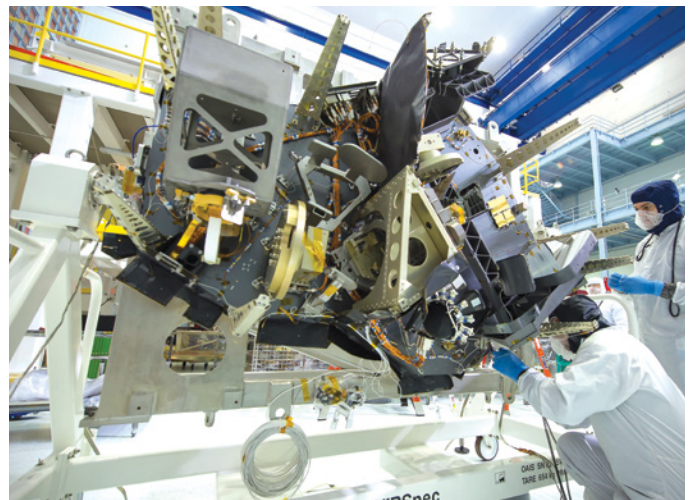
▲ MEGASIZE INSTRUMENTS Engineers prepare the Near-Infrared Spectrograph for acoustic tests.
