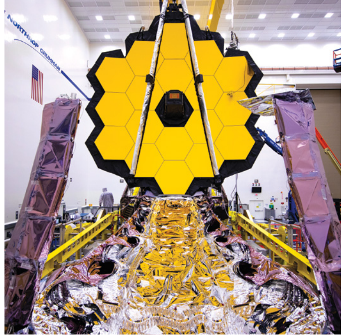
▲ SEMI-DEPLOYED The sunshield lies furled below the unfolded primary mirror. For launch, the shield will fold up and sandwich the mirror.
