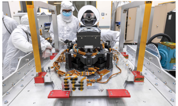
▲ TO DEEP SPACE Team members test the Deep Space Optical Communications experiment in a JPL clean room. The 22-cm primary mirror (center, pointed at camera) will transmit and receive infrared lasers to and from ground stations on Earth. The aluminum base plate will bolt to the Psyche spacecraft.
