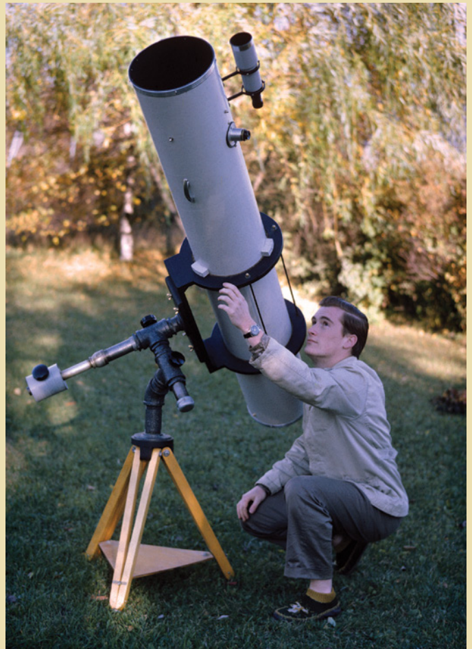
▲ HOMEBUILT PIPE-MOUNTED “CAVE” Coauthor Klaus Brasch with the 8-inch f/7 Newtonian he built in using Cave optics. The scope rides on an iron pipe equatorial mount — something commonly described as a “plumber’s nightmare.” He fashioned other components out of wood, sheet metal, and assorted hardware as suggested in the now-classic Amateur Telescope Making book series.
