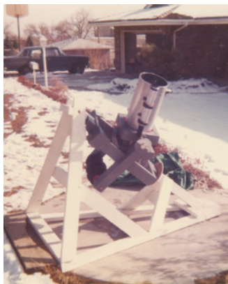
▲ EVOLUTION OF THE 8-INCH At left is the first version of my Newtonian on a Modified English Yoke Mount, while the right-hand photo shows the current incarnation, a fixed-height-eyepiece Dobsonian.
