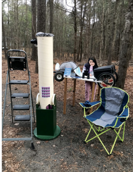
▲ With the addition of screw-on legs, the buggy becomes a chart table.
