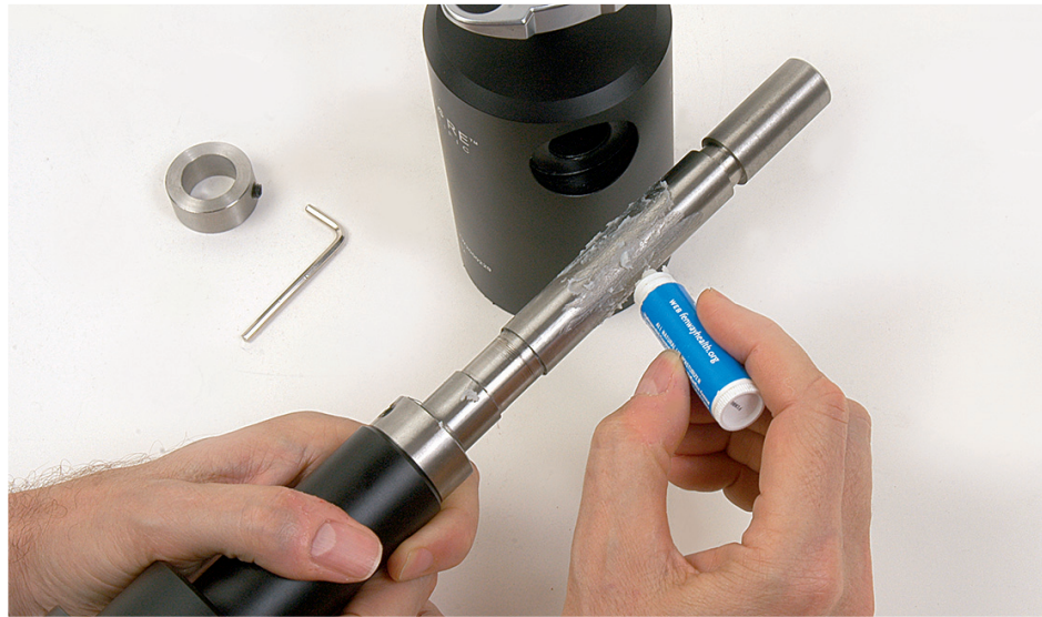
WAX IS THE WAY The motions of this beefy altazimuth mount were greatly improved by cleaning the factory grease off the bearings and applying waxy lip balm instead.
