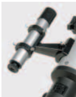
Six of our test scopes came equipped with 5 \times 24 finders. While their single-element objective lenses produced mediocre views, they did function as adequate pointing devices if mated to a two-ring, six-point mount like this one from Meade.
