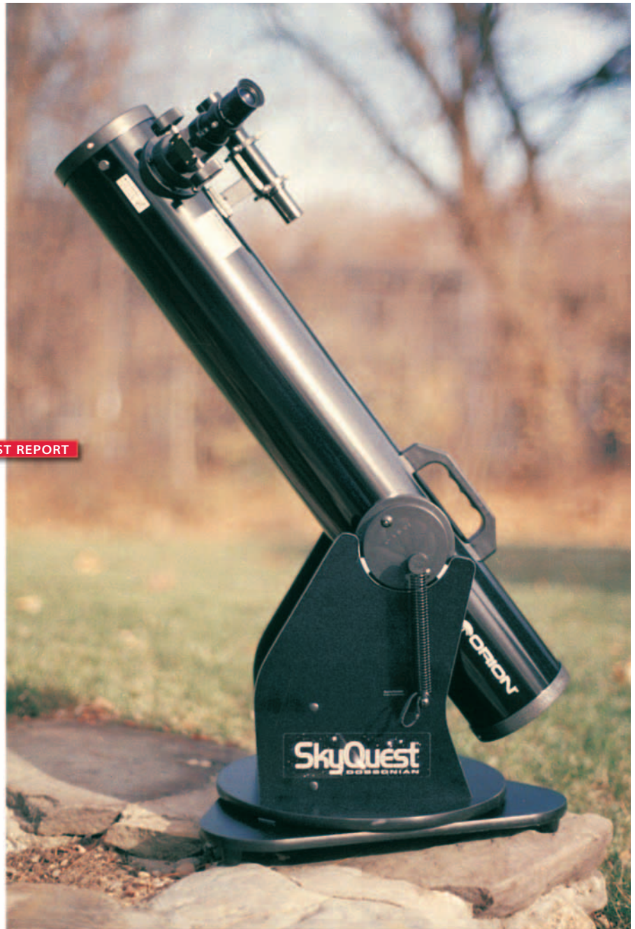
Orion's SkyQuest XT4.5 combines a sleek steel tube with a wooden Dobsonian base in a versatile, 17-pound package. S&T photograph by J. Kelly Beatty.
